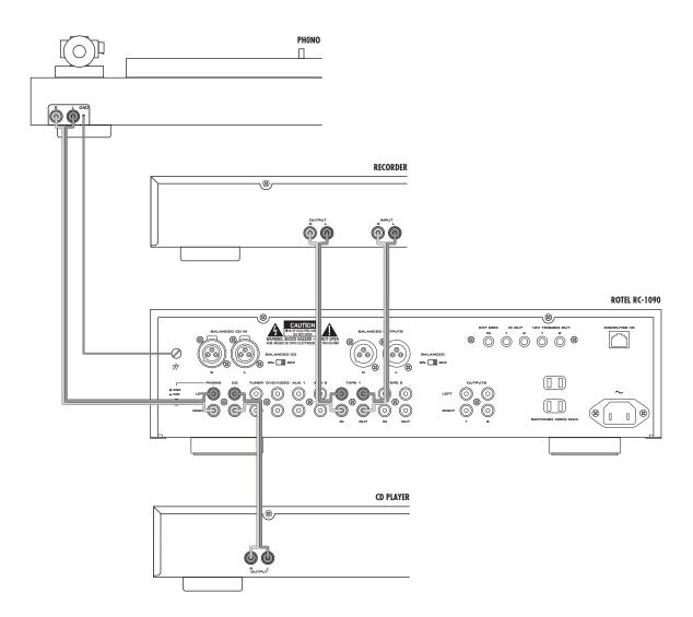
Figure 4: RCA Cable Connections
